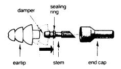
A flat response attenuator attempts to maintain the normal sound quality of instruments and voices but at reduced volume. Two approaches are the ER-20 (shown above) and the ER-15, which uses a custom earmold. By contrast, typical hearing protectors tend to result in a muffled or hollow sound quality.
